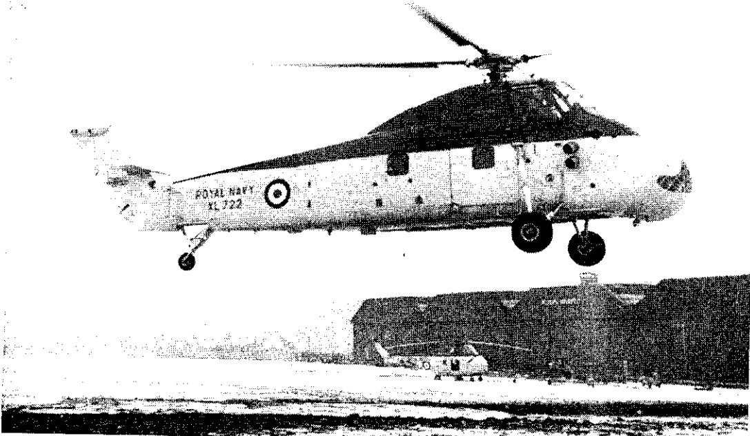
FIG. 9—THE GAZELLE-ENGINED SIKORSKY S.58 WITH THE WESSEX TYPE INTAKE AND NOSE PROFILE
