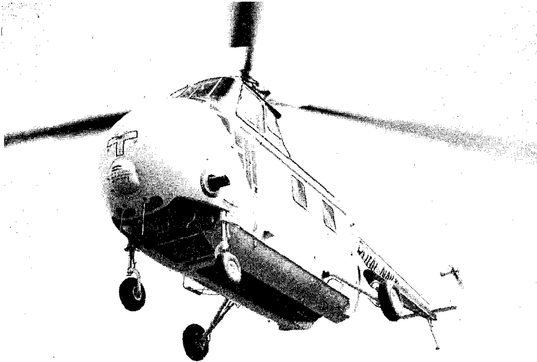
FIG. 4—THE WHIRLWIND H.A.S. MK. 7 HELICOPTER IN FLIGHT. THE WEAPON BAY CAN BE SEEN IN THE FUSELAGE
