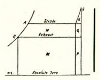
amongst those who visit his engine-testing laboratory. The diagram given by me in my paper on the theta-phi in 1880 makes this very plain. The vertical ordinates here are absolute temperatures, and the area is heat or energy. Without superheating, Carnot's law gives between temperatures A and B.
