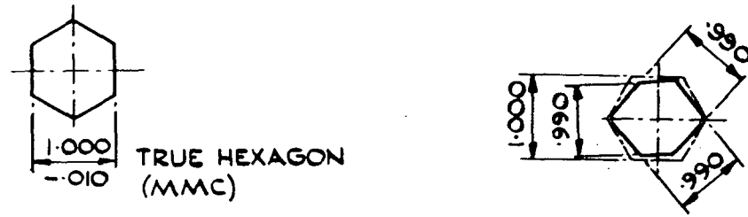
FIG. 2—TYPE OF NOTE USED TO SPECIFY THAT THE FORM IS TO BE CORRECT IF THE FEATURE IS IN ITS MAXIMUM MATERIAL CONDITION
