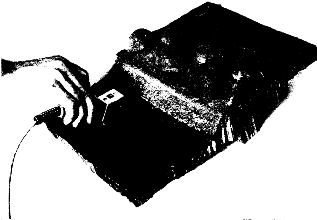
FIG. 8—LOCATION OF PROBE WHEN ULTRASONICALLY TESTING FOR FISSURES AT TOE OF SEAL WELD
