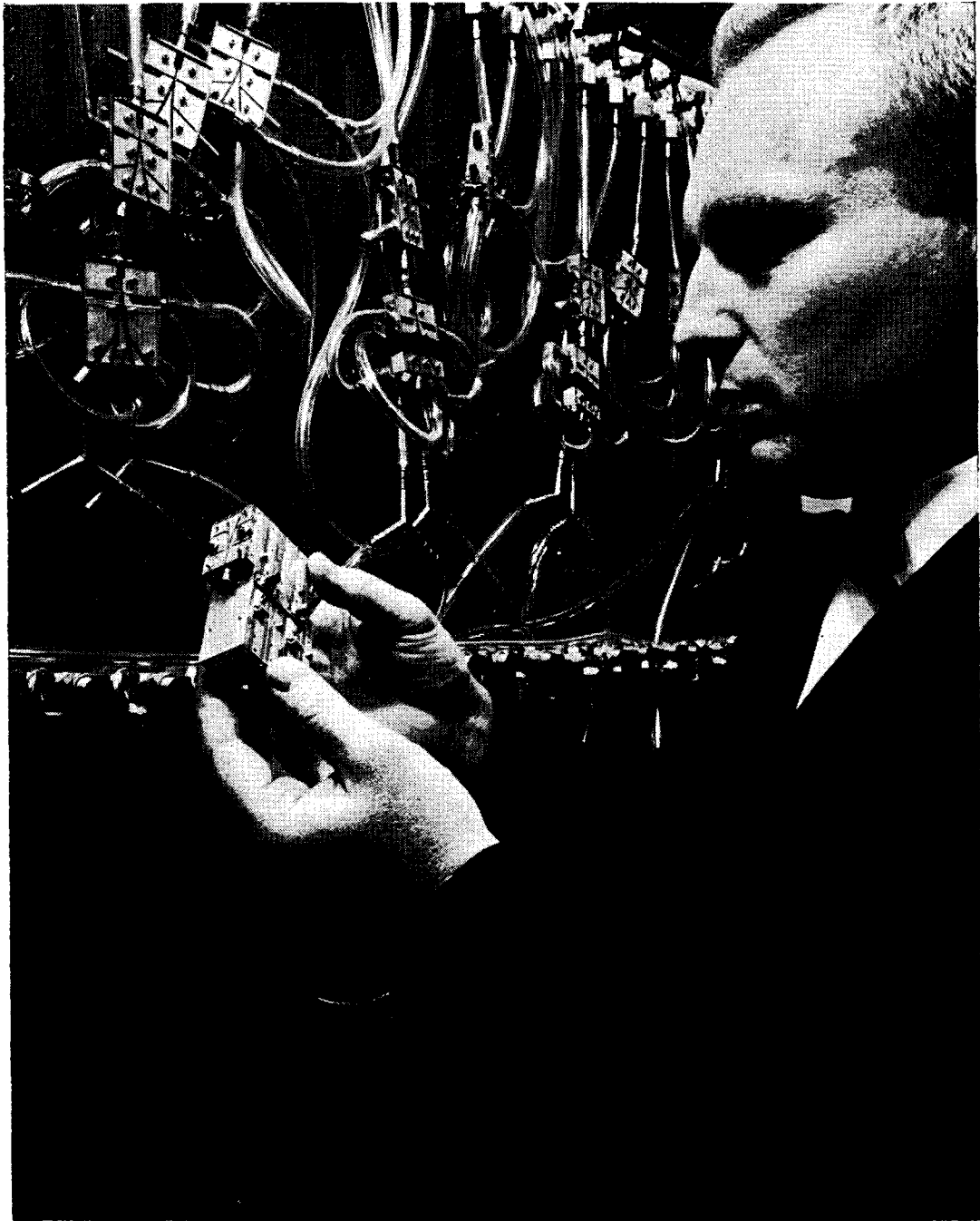
FIG. 11—A FLUIDIC BREADBOARD ARRANGEMENT
