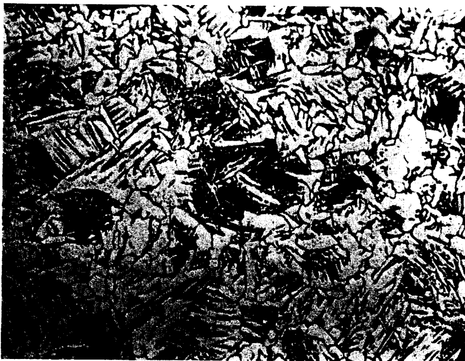
FIG. 6—PHOTOMICROGRAPH OF THE MICROSTRUCTURE OF TUBE A.8, 12 INCHES ABOVE THE BURST ( \times 500 ) The acicular pattern is typical of heating in the region of 860 degrees C, followed by severe quenching from above 700 degrees C.
