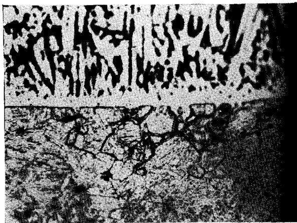
FIG. 9—COPPER INFUSION DOWN GRAIN BOUNDARIES OF STEEL BASE MATERIAL WITH CUPRO-NI DEPOSITED DIRECTLY
