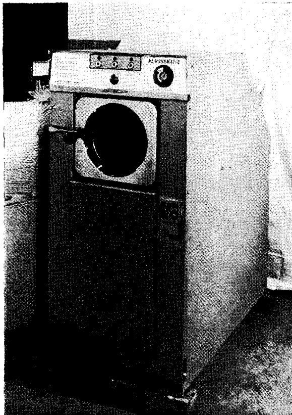
FIG. 2—MODERN WASHER/EXTRACTOR (AUTOMATIC CONTROL)—OUTPUT 24 LB/HR (WASHED AND SPIN-DRIED), FLOOR SPACE OCCUPIED 39½ IN. × 27 IN.
