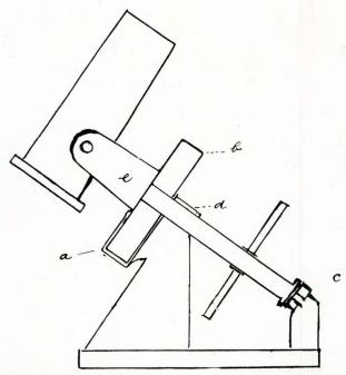
The telescope turns on the axis c, d, e. The hollow steel drum b, concentric with the axis, floats in the hollow tank a. The space is sufficiently filled with mercury to nearly float the whole.
