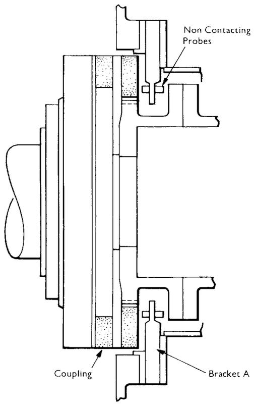
**TYPICAL PROBE MOUNTING BRACKET ASSEMBLY**
