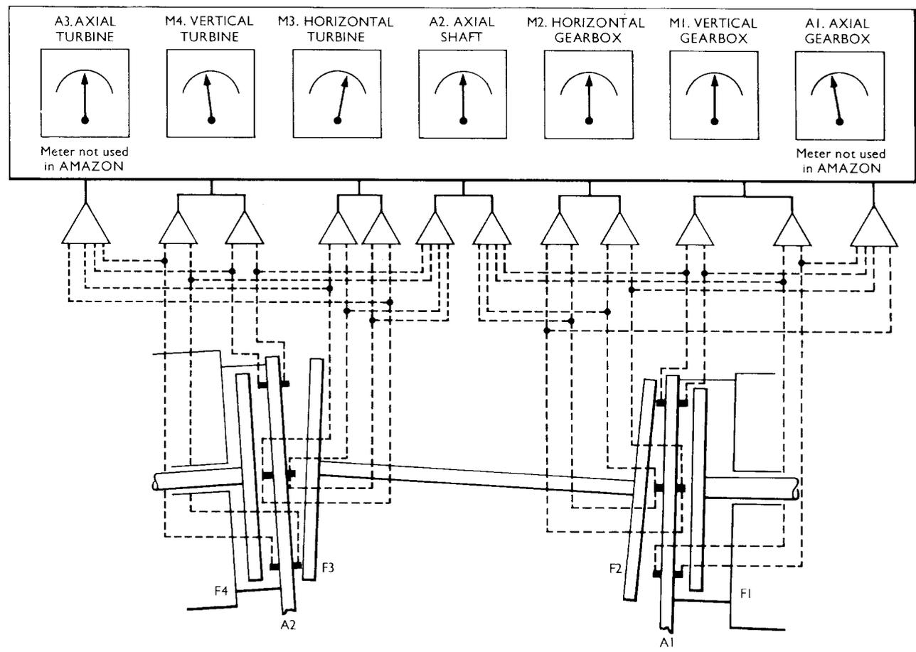
**FIG. 7—SIMPLIFIED SCHEMATIC OF SHAFT ALIGNMENT METER SYSTEM**
