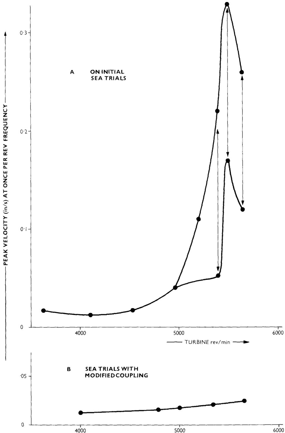
FIG. 6—COGOG OLYMPUS INPUT LINE—VIBRATION LEVELS AT COUPLING SUPPORT BEARING
