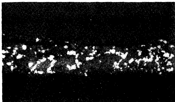
FIG. 4—MICROSTRUCTURE OF BLACK SCALE SHOWN BY ARROW 2 IN FIG. 1. TIN OXIDE LAYER IS APPROX. 0.002 IN. THICK
