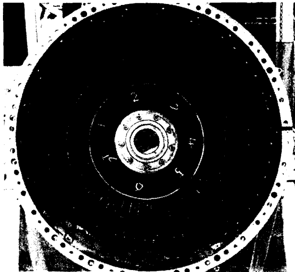
FIG. 8—TYNE OUTLET GUIDE VANE: FRETTING OF ROOT PLATFORMS
