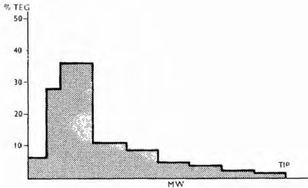
FIG. 6—GP FRIGATE ENERGY CONSUMPTION (PROPULSION AND AUXILIARY LOAD)
