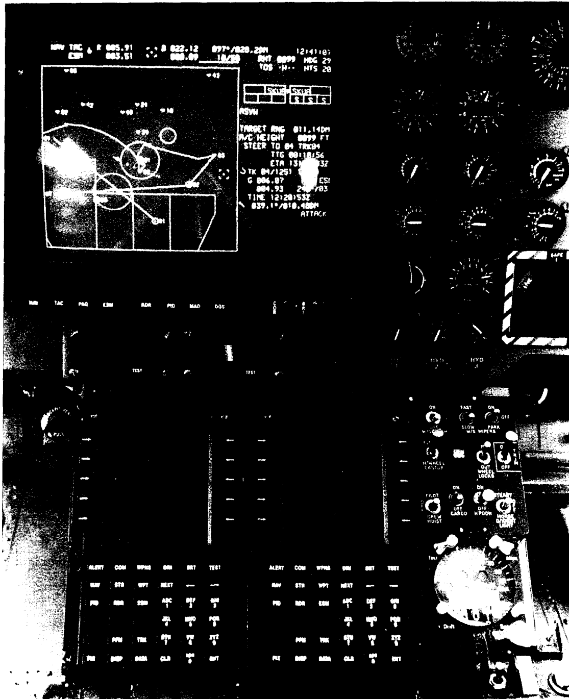
FIG. 4—CLOSE-UP VIEW OF THE LYNX Mk.3 (CTS) COCKPIT INSTRUMENT PANEL SHOWING THE TACTICAL SITUATION DISPLAY (TOP LEFT) AND THE TWO CONTROL DISPLAY UNITS (BOTTOM)
