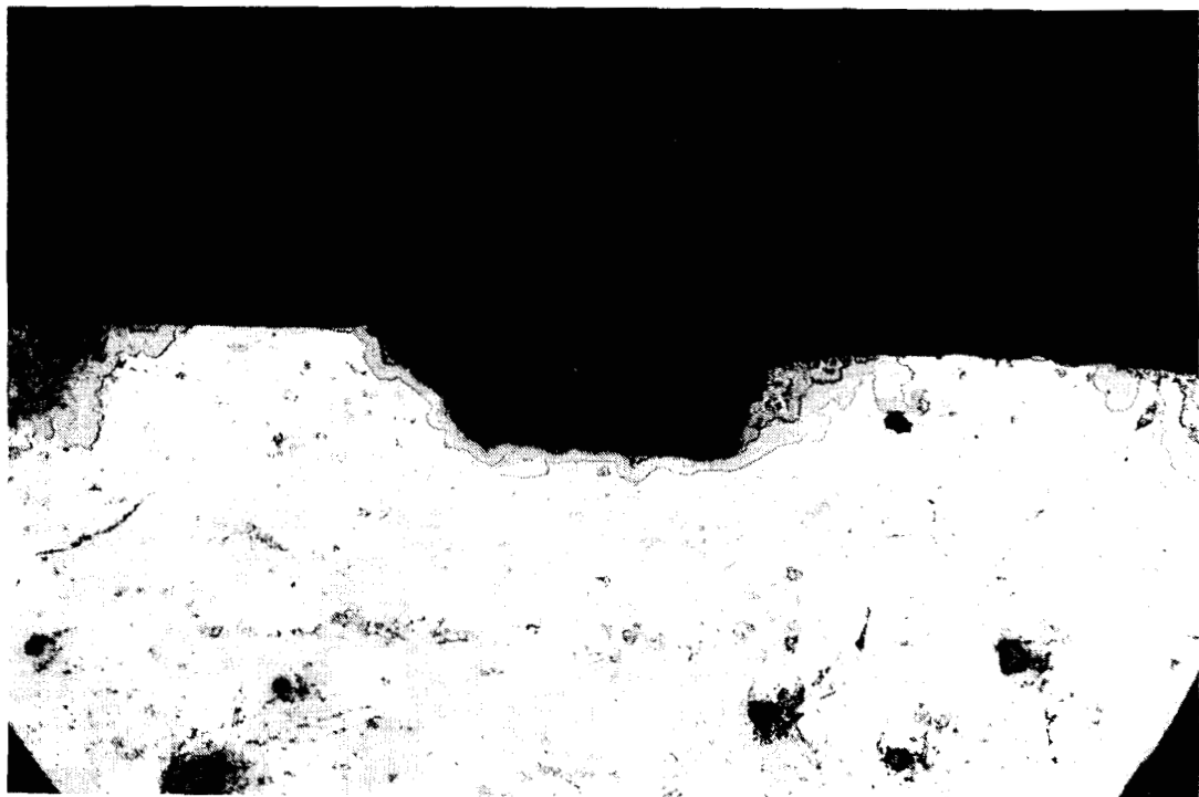
SECTION THROUGH RILLENLAGER GROOVE SHOWING LOSS OF OVERLAY
