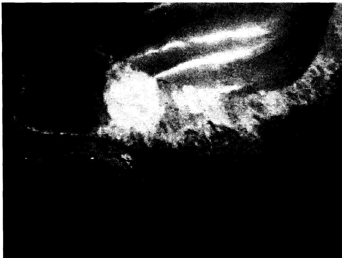
FIG. 37—FULL SCALE ROOT CAVITATION ON A HIGH SPEED PROPELLER
