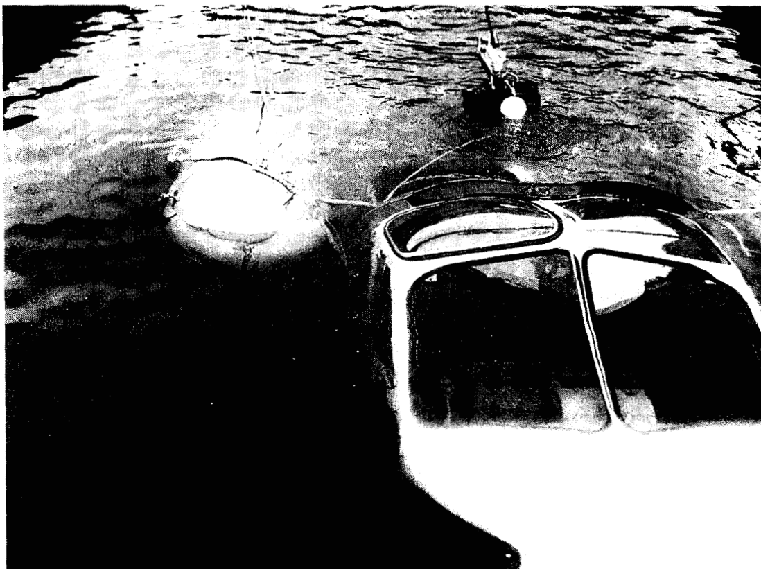
FIG. 4—DEVELOPMENT TRIALS OF WASP FLOTATION GEAR BY THE FAIREY AVIATION DIVISION OF WESTLAND AIRCRAFT, AT HAYES IN NOVEMBER 1964
