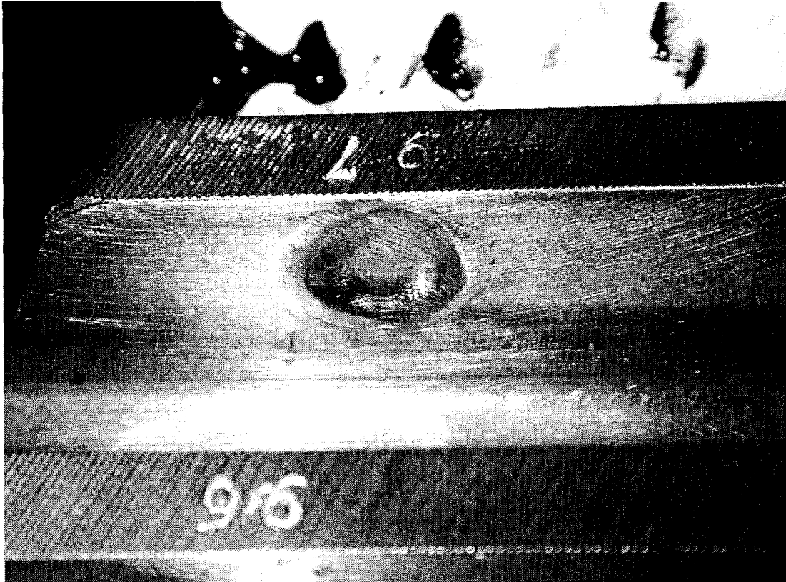
FIG.5 – DRESSING TO REMOVE TOOTH SECTIONS AND AREAS OF PITTING.
