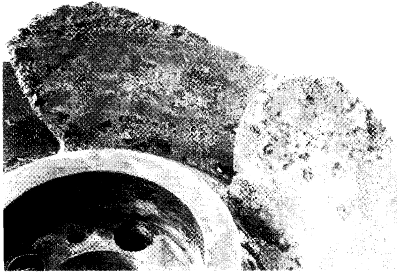
FIG.3 CORRODED NAB IMPELLER
