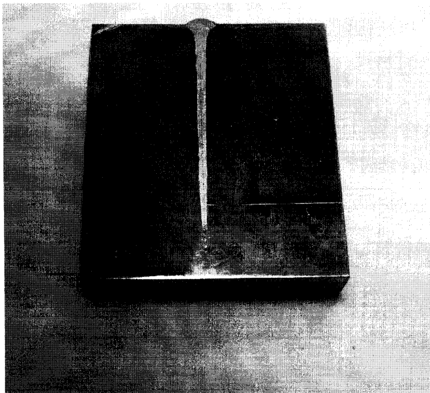
FIG.5 MACRO SECTION THROUGH A TEST EB WELD
