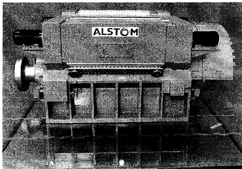
FIG.8 – MODEL OF ESTD 20 MW AIM
