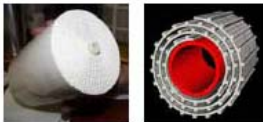
FIG.3 – PICTURE OF RPC REMOVED FROM STORAGE CANISTER; DIAGRAM OF A SECTION OF RPC SHEET, RIBBED FOR TUNED AIR FLOW
