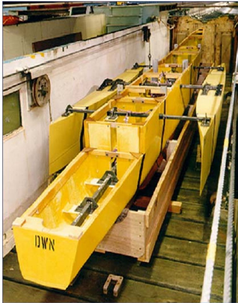
FIG.30 - SEGMENTED MODEL (COURTESY OF QINETIQ)
