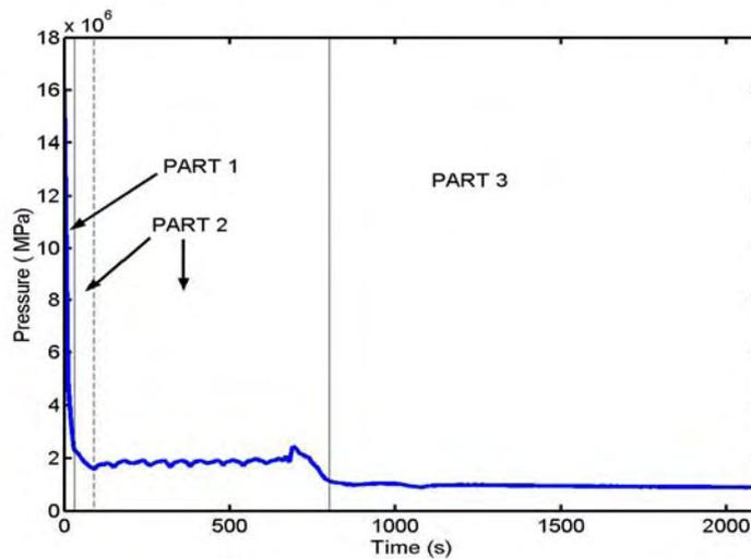
FIG.13 - PRESSURE FOLLOWING BREAK IN THE CONNECTING PIPE TO THE PRESSURISER (50 MM), INITIAL POWER 50 MW, ECCS FULLY AVAILABLE
