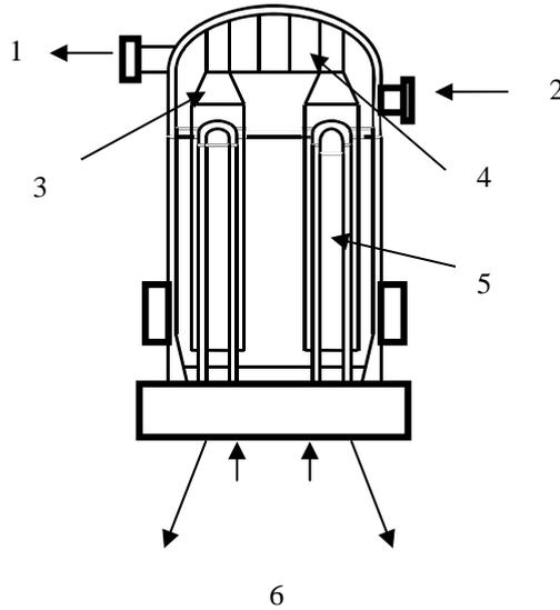
FIG.11 - STEAM GENERATOR LAYOUT
