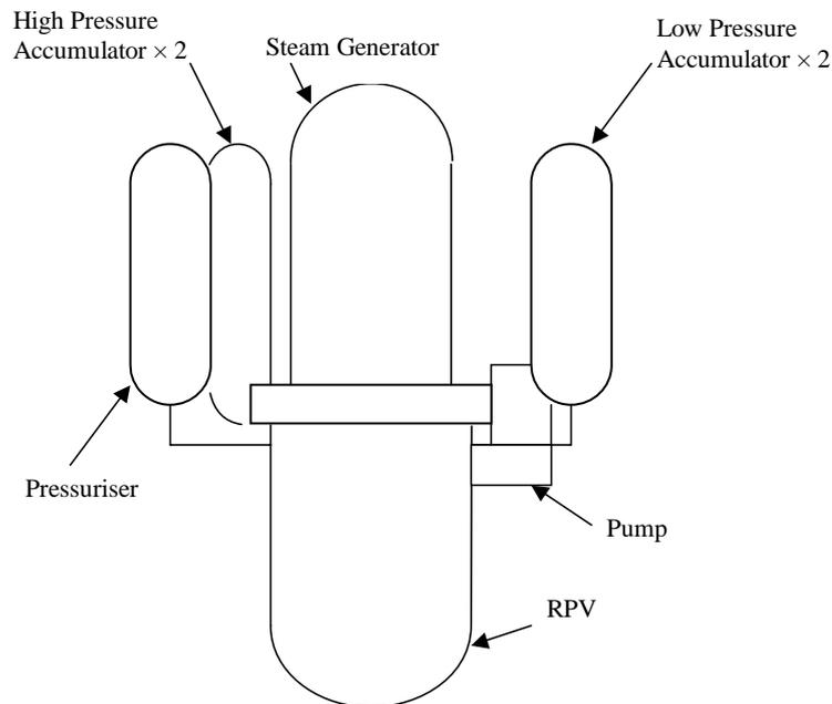
FIG.1 - INTEGRATED PLANT LAYOUT, SHOWING SG ABOVE RPV, PRESSURISER AND ECCS ACCUMULATORS
