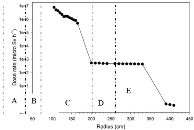
FIG.10 - SECONDARY GAMMA DOSE RATE MID CORE PLANE
