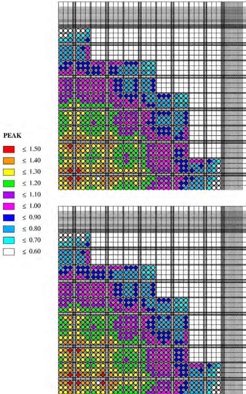
FIG.5 - POWER PEAKING FACTORS AT SOL (TOP) AND EOL (BOTTOM) FOR FINAL CORE CONFIGURATION
