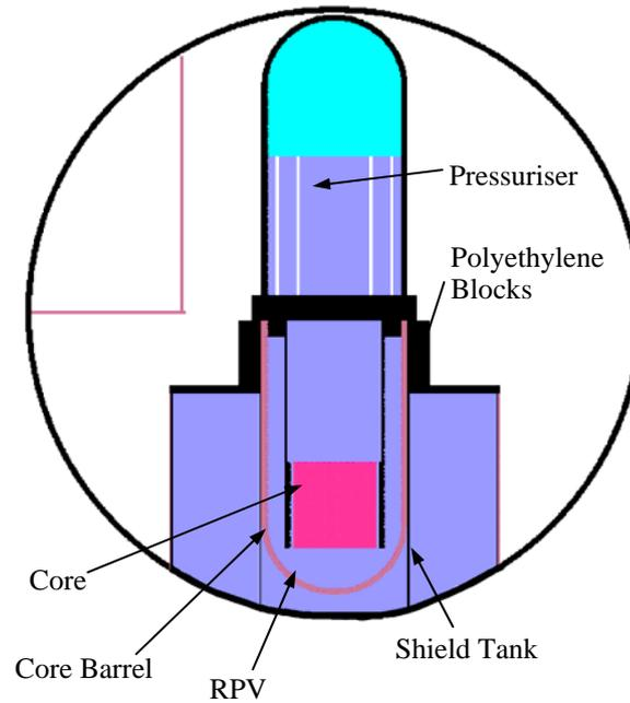
FIG.8 - ELEVATION OF THE CORE AND PRIMARY SHIELD
