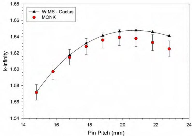
FIG.2 - VARIATION OF  $K_{\infty}$  WITH PIN PITCH
