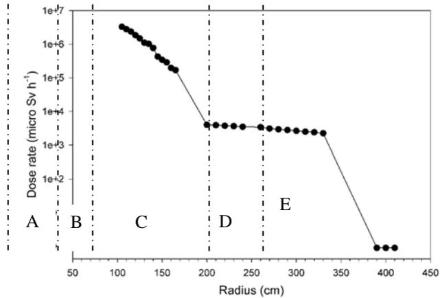
FIG.9 - PRIMARY GAMMA DOSE RATE MID CORE PLANE,
