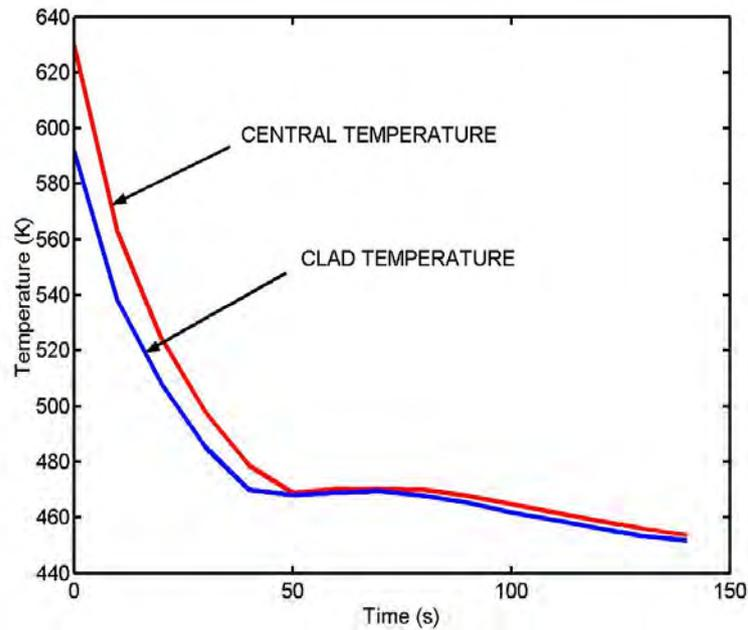
FIG.14 - FUEL AND CLAD TEMPERATURES FOLLOWING A BREAK IN THE SURGE LINE. INITIAL POWER 15 MW, HALF ECCS AVAILABLE
