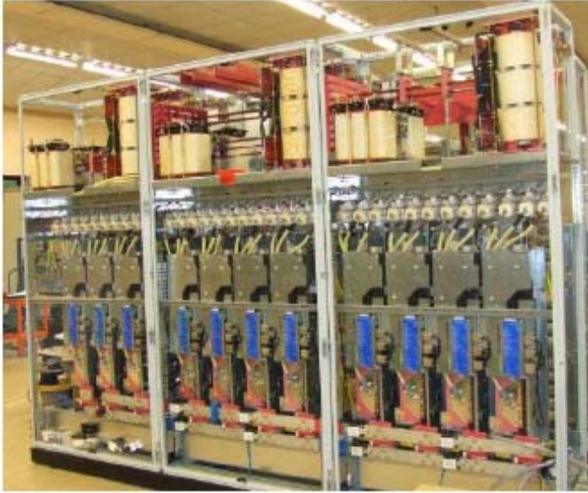
FIG.4 - 7.5MVA EMKIT CONVERTER
