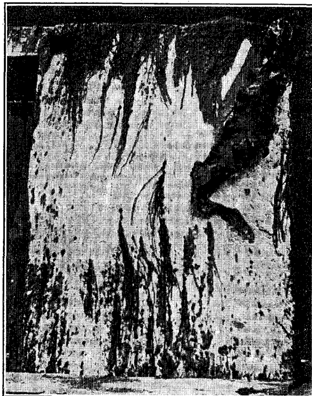
FIG. 6.—A TEST PANEL EXPOSED ON A RAFT IN THE MENAI STRAITS, CAERNARVON, FOR 10 MONTHS. THE PAINT HAS WORN THIN IN THE BRUSH MARKS AND ALGAE HAVE GROWN IN THE LOCALLY NON-TOXIC "TROUGHs"
