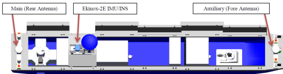
Figure 2: Positions of the sensors on the body frame.
