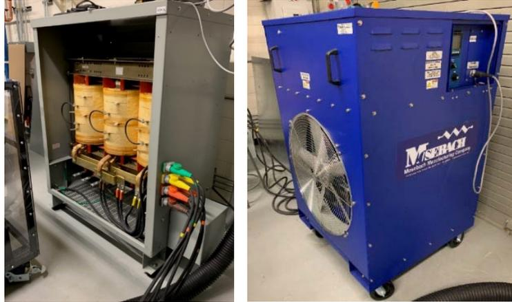
Figure 6: Photograph of the 500 kVA - 4160 VAC / 480 VAC step down transformer installed in the laboratory (left) and of the Mosebach 350 kVA - 480 VAC resistive electronic load installed in the laboratory (right).
