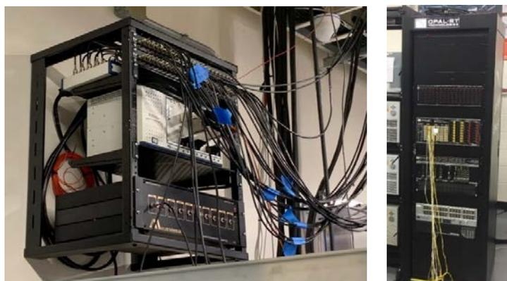
Figure 14: Photograph of the NI PXI chassis and OPAL-RT, respectively.
