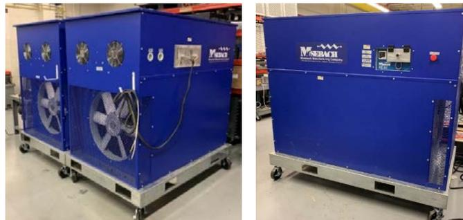
Figure 9: Photograph of the two 6 kVDC – 150 kW resistive loads (left), and 12 kVDC – 100 kW resistive load (right).
