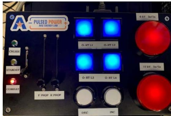
Figure 16: Photograph of the user control box designed and developed for interfacing with the testbed.
