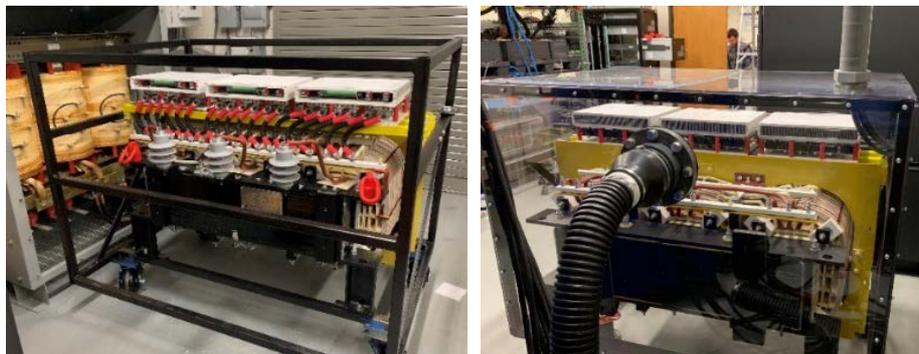
Figure 7: Photograph of the 225 kW, eighteen - phase transformer and thirty-six pulse AC/DC rectifier within the custom enclosure fabricated for safety and for forced air cooling. The transformer is below and the white rectifiers are seen above it.
