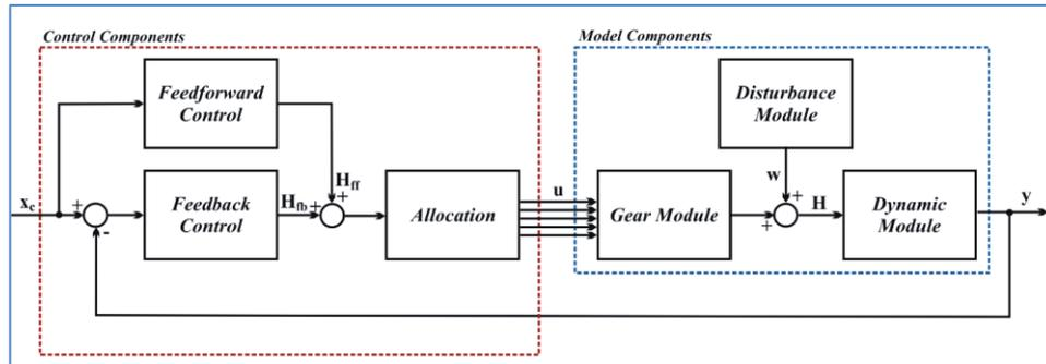
Figure 5: Modular velocity control loop structure
