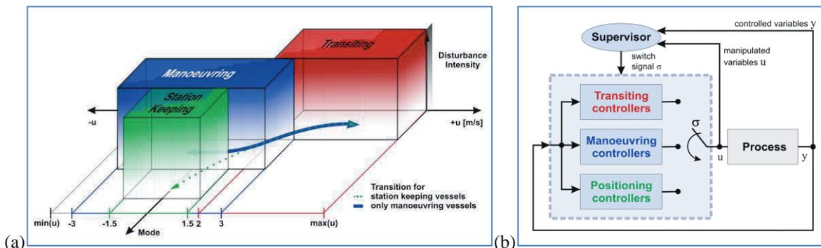
Figure 4: (a) Vehicle motion modes (b) Scheme of a switching control system
