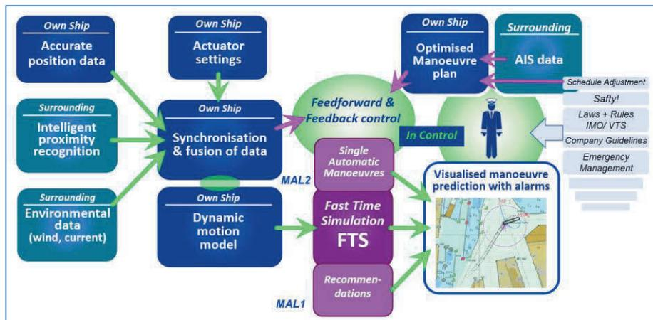
Figure 2: Necessary infrastructures for manoeuvre assistance – MAL 1 and partial manoeuvre automation – MAL 2
