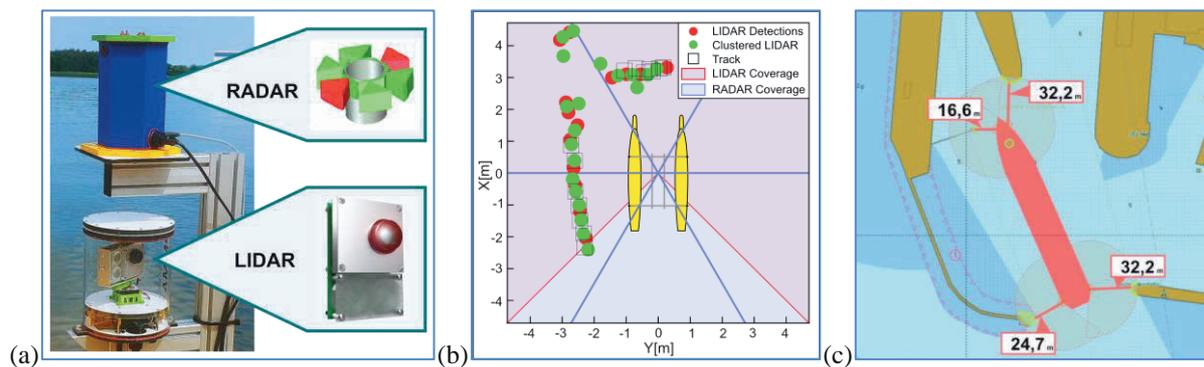
Figure 3: (a) Radar-lidar-system installed on USV, (b) Scatterplot of proximity distances around the USV, (c) Concept of presentation of proximity distances on larger vessels in ENC
