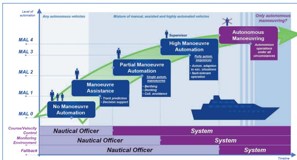
Figure 1: Automation levels of manoeuvring of maritime surface vehicles
