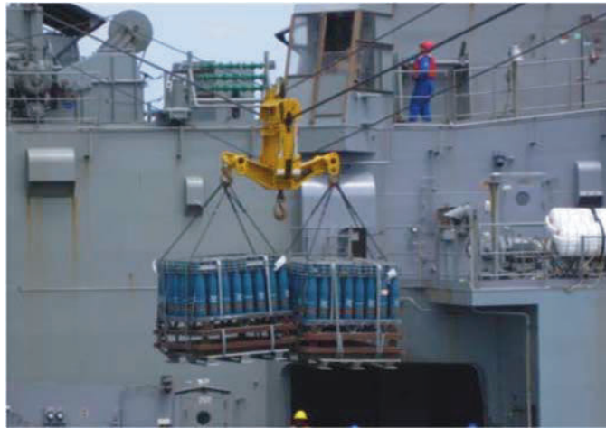
Figure 9 - Heavy E-STREAM trolley transferring 12,000lb test load during at sea qualification trials (McLachlan, 2014)
