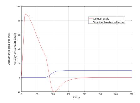
Figure 5: Motion of the azimuthal system commanded by the adaptive PD control.
