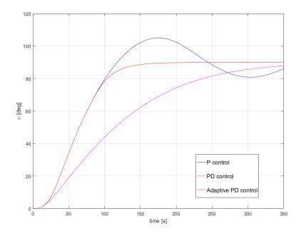
Figure 4: Orientation evolution under the control of the adaptive PD regulation scheme.
