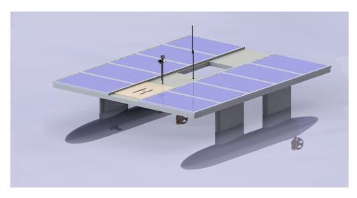
Figure 1: Rendering of the SWATH platform.
