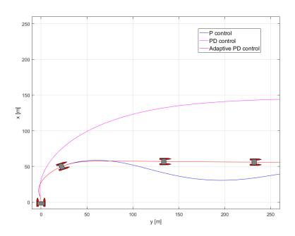
Figure 3: Motion generated by the thrust and course control system.
