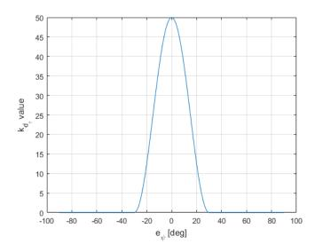
Figure 2: The adaptive derivative coefficient function.
