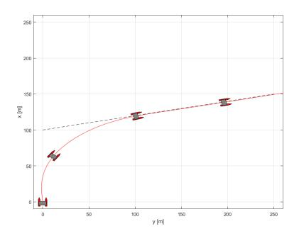
Figure 7: Path-following guidance along a rectilinear line.
