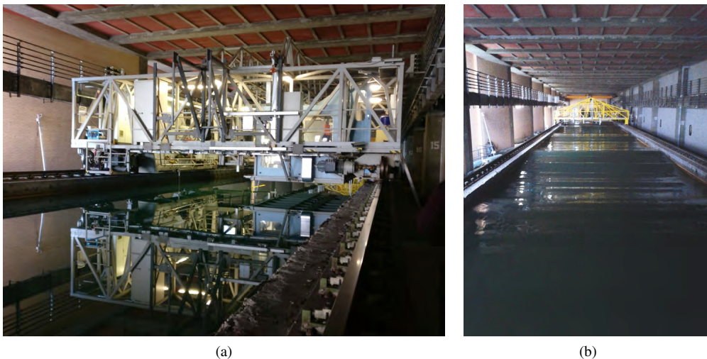
Figure 3: Tank no. 2 facilities. (a) The carriage system. (b) View of the tank while the wave generator is in motion.
