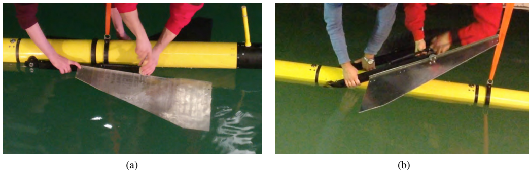
Figure 6: Wing sections in the two mounting directions. (a) Right Side Up mounting direction. (b) Upside Down mounting direction.
