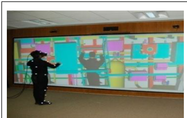
Figure 7:- The inspection of compartment at the VR lab at M/s MDL, India. (Source https://mazagondock.in/Design-Facilities.aspx )
