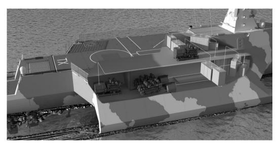
Figure 5 - Illustration of the CODLAD propulsion system within the Tx hull-form
