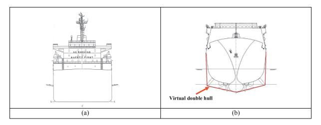
Figure 5: Comparison of Cross-Sections of Typical Merchant Ship (a) With Surface Combatant (b)
