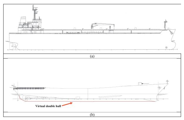
Figure 4: Comparison of Profile of Typical Merchant Ship Hull (a) With Surface Combatant (b) (note uniform baseline of merchant hull and the absence of projections)
