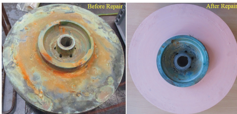
Figure 14: Repair and preservation of a HPSW pump impeller
