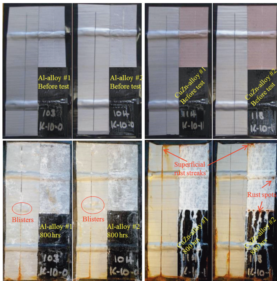
Figure 11: Accelerated salt-spray (ASTM B117) corrosion testing of Al-alloy and CuZn-alloy LP-CMS coatings
