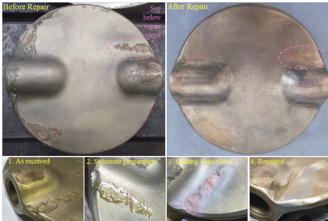
Figure 13: Repair and restoration of a seawater valve disc with LP-CMS coatings
