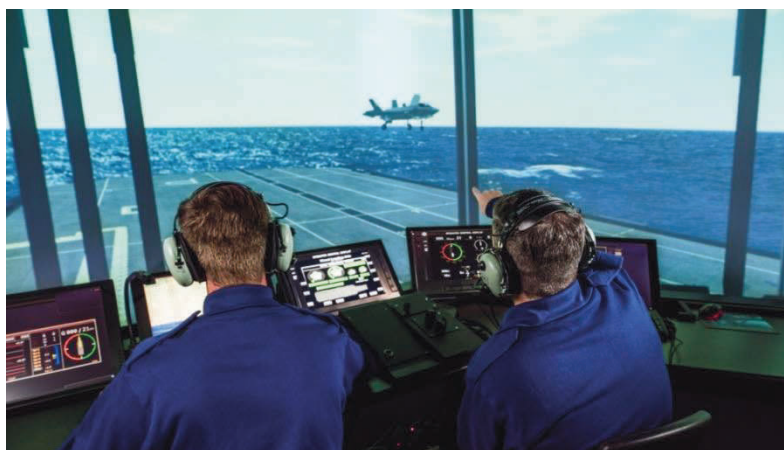
Figure 12: F-35/QEC simulation facility at BAE Systems Warton, showing inside of networked FLYCO simulator
