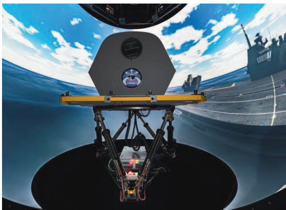
Figure 10: F-35/QEC simulation facility at BAE Systems Warton, showing motion system and dome
