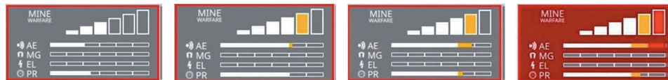
Figure 8: The indicator shows the ship’s susceptibility to a threat. Above figure show the susceptibility to a mine threat at high ship speed. Four signatures (acoustic, magnetic, electric and pressure) can contribute to the mine threat susceptibility as shown below the strength indicator. In this case the main contributor is the emitted acoustic noise (shown by the horizontal bar), a secondary is the pressure signature.
