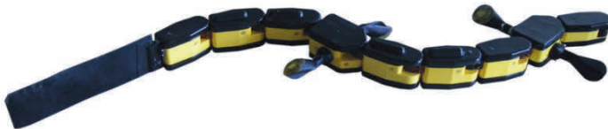
Figure 12 - Salamandra robotica II. It can swim, crawl, and walk. Has been shown to be robust against damage, as this robot could lose parts of its body and still be able to walk.
