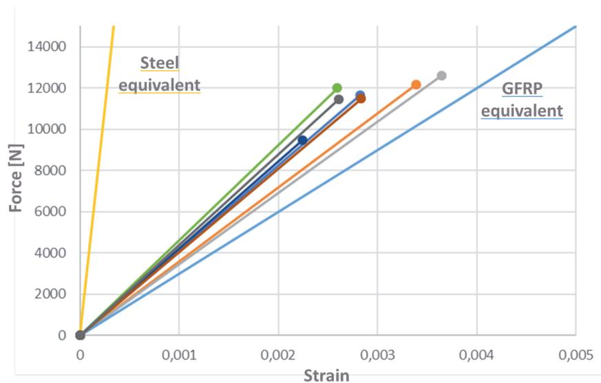
Figure 6. Representative Force-Strain curves. Note: Curves with dot mark the FAUSST specimens at first failure load. Steel and GRFP (43Vol.% of Bi-directional E-Glass fibres) are displayed for comparison.
