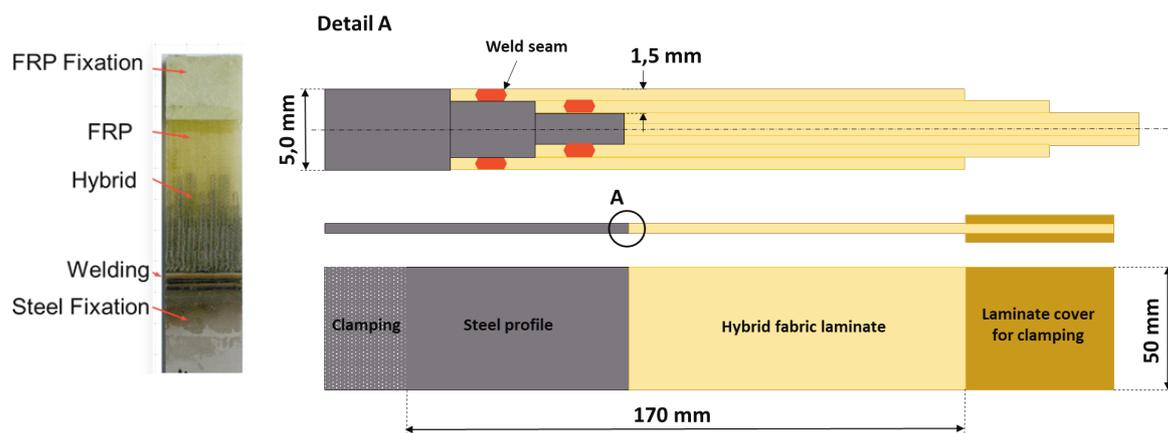
Figure 5. Specimen geometry and welding details. Left side: photo of specimen. Right side: schematic of layout. Note: specimen not scale
