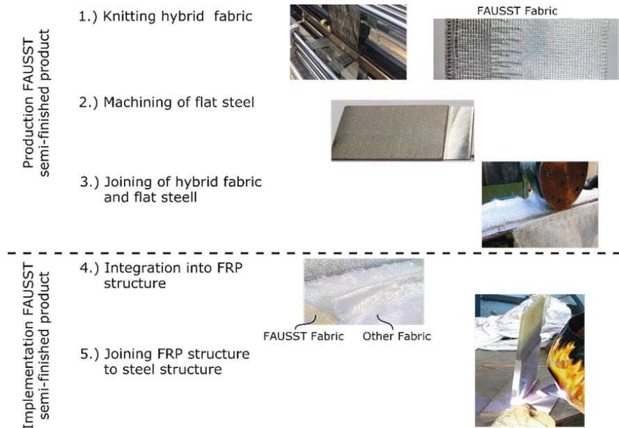
Figure 2: Fabrication and installation process of FAUSST
