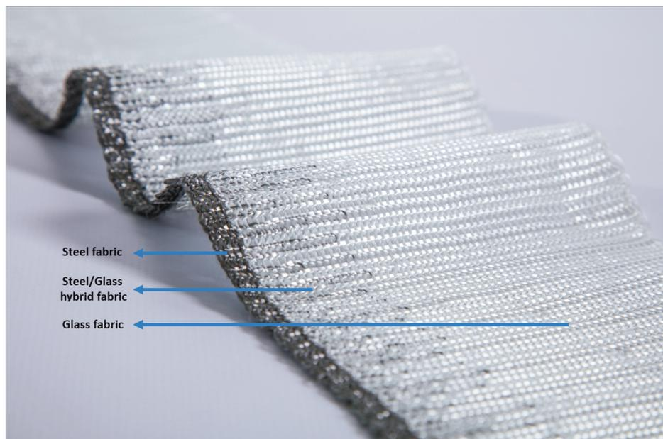
Figure 1: warp knitted hybrid fabric from steel and glass fibres
