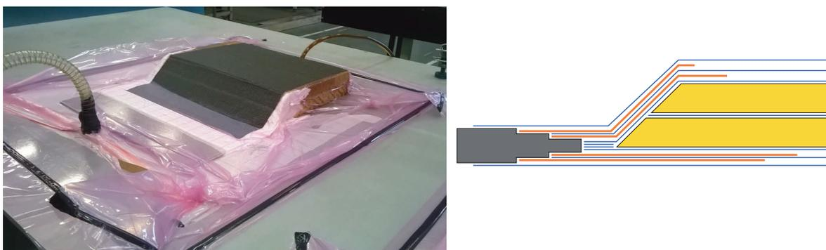
Figure 4: Left side: vacuum infusion of demonstrator. Right side: Layout of FAUSST integration - Grey=steel bar; red=hybrid fabric of FAUSST; yellow=core material; blue=glass fibre plies
