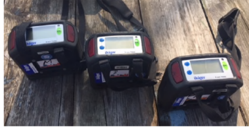
Draeger X-am 7000 CO 2 Measurement Gauges
