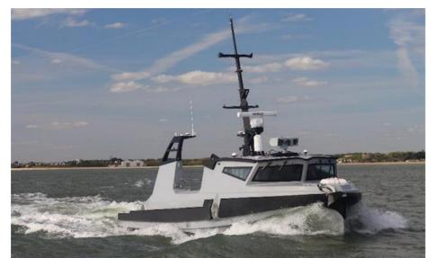
Figure 5. L3 Technologies Mine Countermeasures (MCM) Autonomous Vehicle for Thales UK
