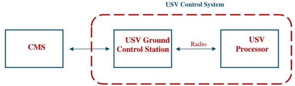
This architecture allows the CMS to send commands to the unmanned surface vehicle's ground control station which then converts the message to a format readable by the unmanned surface vehicle processor.
