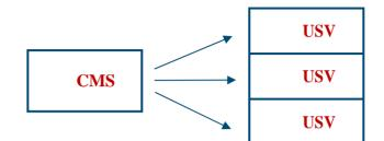
The above scenario would work well when the off-board systems are within good communications range of the mothership. Once out of communication range, the behaviour of the USV will be dependent on the autonomous control software. An example behaviour could be that the USV returns to the last known location where it was receiving communications, known as the Last Response Engine.
