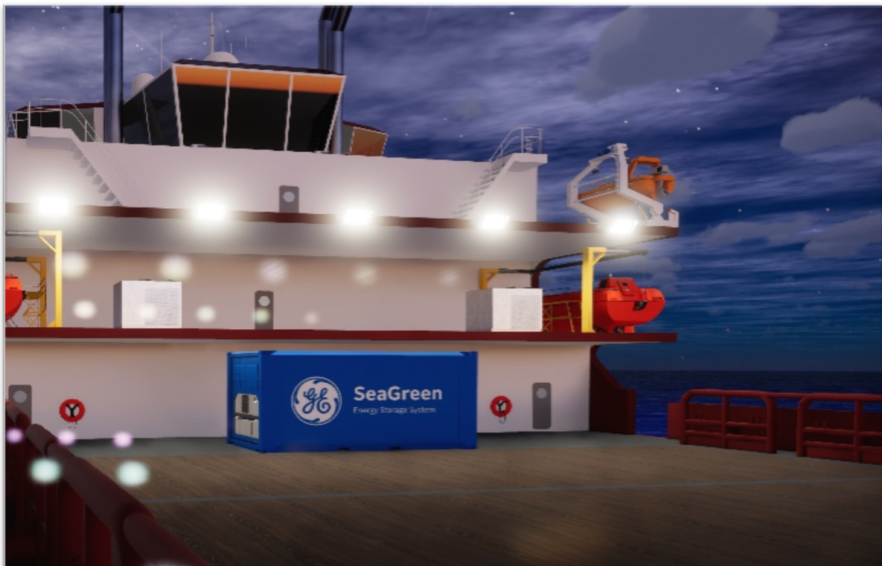
Fig.3 Self Contained Retrofittable Deck Mounted Energy Stores
