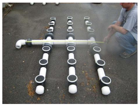
Photo 17 – Diffuser grid of 18 coarse bubble puck diffusers
