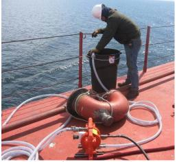
**Photo 10 - Perforated hose setup on deck during dye study** *Note: Appropriate PPE should be used when handling hazardous chemicals.*
