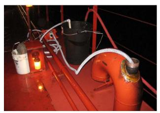
Photo 9 - Dosing setup on deck
