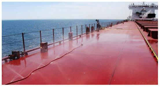
Photo 19 - Testing the spray pattern of the perforated hose
