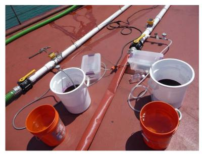
Photo 15 - Nozzle equipment on deck: hoses, valves, meters, chemical injection equipment
