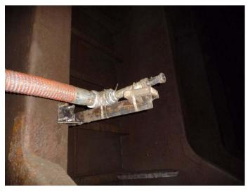
Photo 14 - Nozzle mounted to ship's structure in tank in parallel nozzle arrangement
