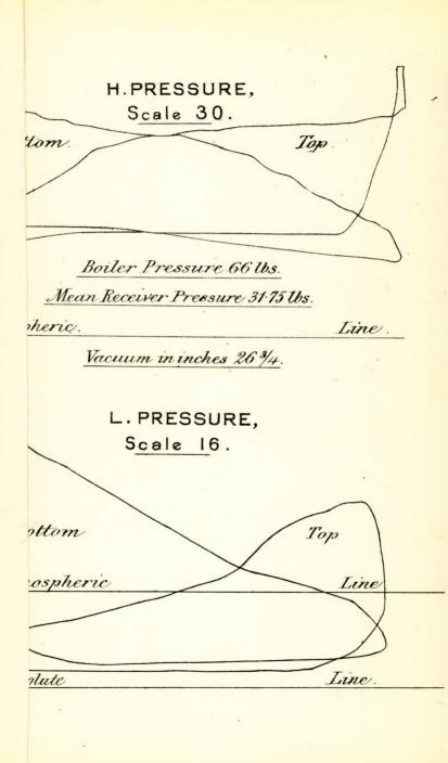
the H.P. is increased almost inversely as the cut off fraction. In this way the power developed in the high is reduced and the initial pressure in the low is increased.
