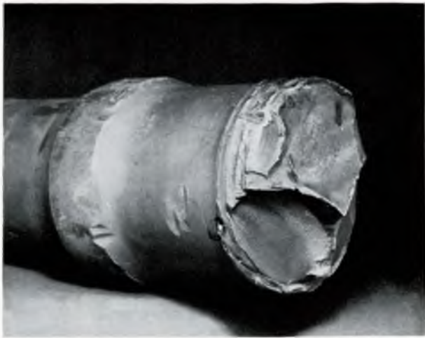
FIGS. 16(a) (above) and (b) (right)—Compound fatigue fracture of 4-in. diameter bottom-end bolt
