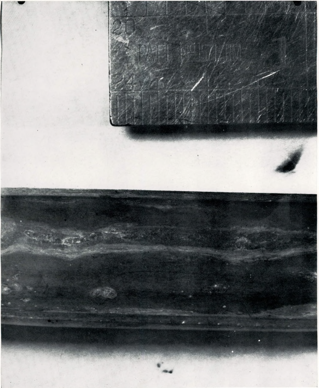
FIG. 14.—ENLARGED VIEW OF GENERAL DETERIORATION OF ALUMINIUM-BRASS TUBE
