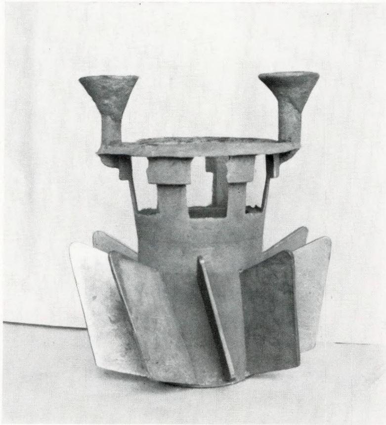
FIG. 13—Part of oil burner in S.G. iron with casting heads attached By courtesy of Mario Pensotti, S.p.A., Milan, Italy
