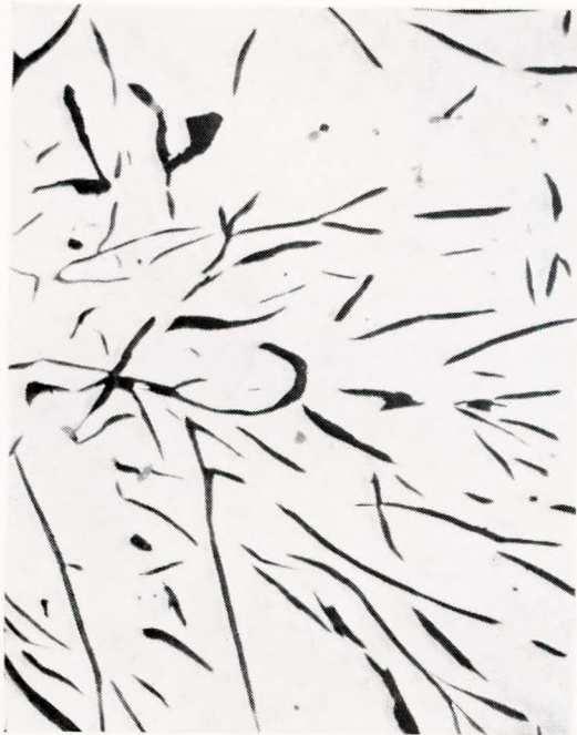
FIG. 1—Unetched. Graphite flakes in grey cast iron × 100
