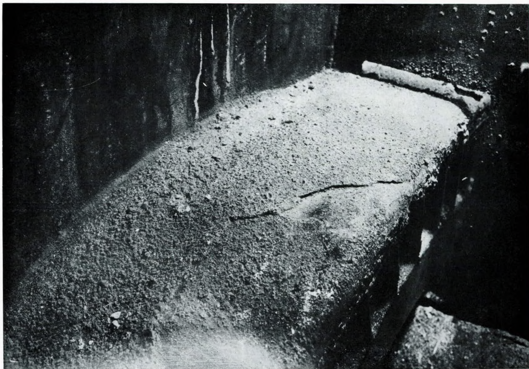
FIG. 3.—STATIONARY BLADING AT GAS INLET SIDE
