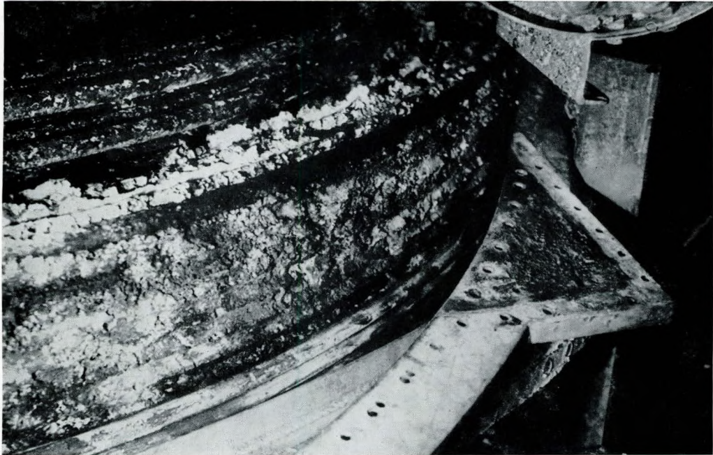
FIG. 1.—TYPICAL DEPOSITS IN THE TUBE NEST OF A BOILER OF A BATTLESHIP AFTER OPERATION WITH CONTAMINATED FUEL.
