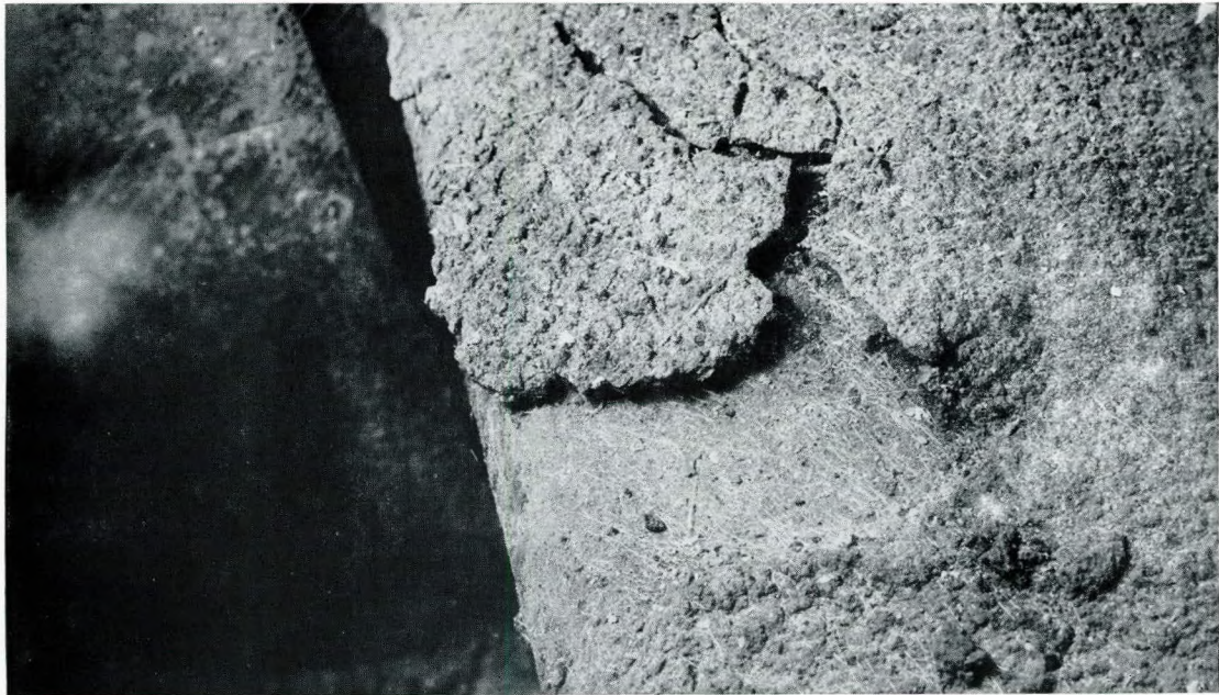
FIG. 2.—PHOTOGRAPH SHOWING THE AMOUNT OF DEPOSITS WHICH HAVE ACCUMULATED AT THE INLET OF A GAS TURBINE. CHEMICAL ANALYSIS OF THE DEPOSITS IS AS FOLLOWS:
