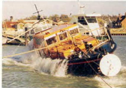
The future RNLB Marine Engineer during successful self-righting trials at Cowes, Isle of Wight,
