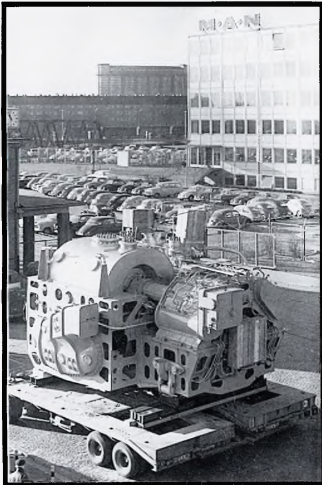
Fig 21: Hamburg Class machinery; West German destroyer powered by 2 x 34 000 shp MAN turbines, 900 lb/in 2 /850°F (Note packaged unit construction)
