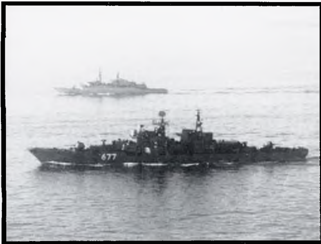
Fig 20: Soviet Sovremenny Class destroyer powered by 2 x 55 000 shp steam turbines
