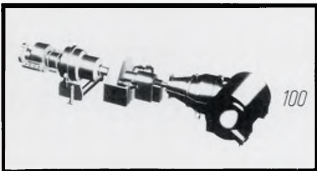
Fig 8c: Stal Laval progress; VAP, 1981, 126 bar/600°C/ 600°C (Only built in prototype form)
