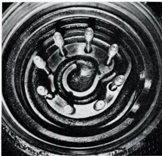
FIG. 6—Piston cooling space of oil cooled piston of a slow speed crosshead engine—One year's operation with an additive type system oil
